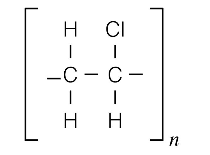
Third most widely produced polymer plastic Rigid form: pipes, door and window frames, ... Flexible form: electrical cable insulation, flooring, ...
